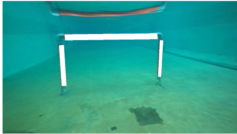
Fig. 9. Full feature detection stack applied to a recording of the gate. Note that compared to Figure 17, the outliers have been filtered out, and only the gate is detected.
