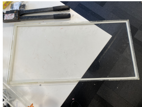
Figure 4: Electrical housing lid with glued EDPM seal.
