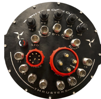
Fig. 6. Laser engraved connector lid for the electronics housing.
