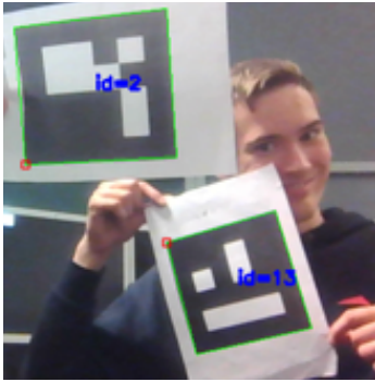
Fig. 12. ArUco detection and identification
